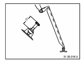
Inspection dimension (C) for accelerator pedal, refer to Technical Data.
