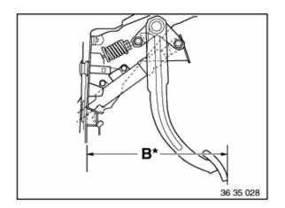
Inspection dimension (B) from underside of pedal to face wall for: Clutch pedal (dimension B), refer to Technical Data. Brake pedal (dimension A), refer to Technical Data.
